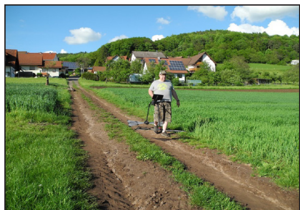
Figure 14: Vertical GPR measurements on the mine's rooftop, in 2D mode, and using triangular antennas.
