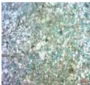
Figure 1: Core sample C thin section image using x5 magnification which shows high porosity.
