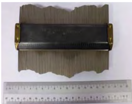
Figure 1: The 15 cm comb profiler or Barton comb for the determination of the joint roughness coefficient, JRC.
