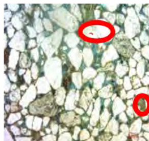
Figure 2: Core Sample A thin section image using x5 magnification shows low porosity, compared to core sample C due to compaction(a) and some of iron oxide(b).
