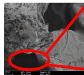
Figure 6: SEM image shows a pore space in between the grain.
