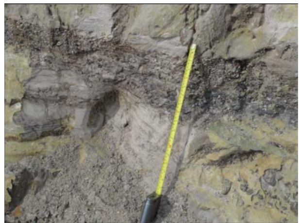
Figure 8: Clay clast and quartz pebble bed at the bottom of a cross-bedded sandstone unit, Tukau Formation, Bakam quarries. This bed is comprised of 60% irregularly-shaped clay clasts and 4% quartz and hard rock conglomerate. It could be a flash-flood deposit.
