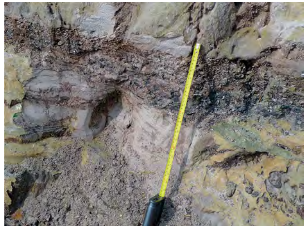
Figure 4: Micro-conglomeratic bed at the bottom of cross-bedded sandstone unit, Tukai Fm. This bed is formed of 60 % irregularly shaped clay clasts and 40 % quartz and hard rock conglomerate.
