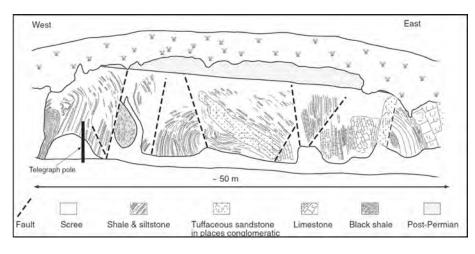
**Figure 3:** Sketch of north side of road-cut at Jengka Pass (from Lee, 2009).
