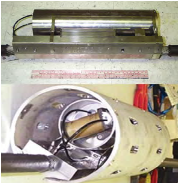
Figure 4: Sensor pad assembly showing a side view of geophone housing on sensor pad base (upper), and an end-on photo of the protective housing shows a hydrophone mounted in the pad (lower).
