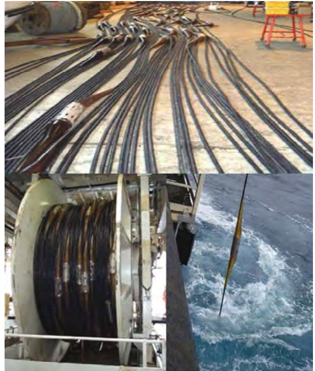
Figure 5: Optical seabed array being prepared in the warehouse (upper), on a deployment reel (lower left), and during deployed (lower right).
