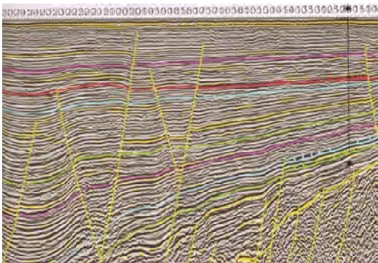
Figure 1: Fragment of a regional seismic line across the Malay basin. Some of the deeply rooted regional faults reach up very close to the sea bed.
