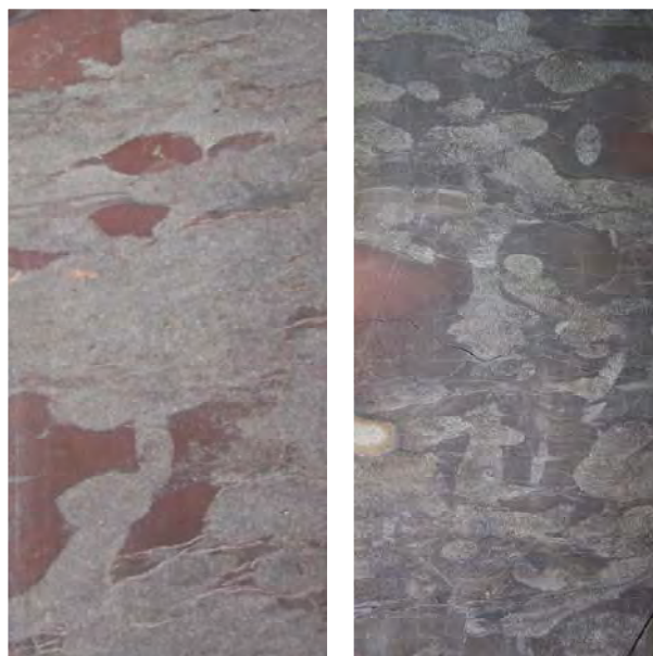
Figure 1: Two core intervals which represent part of the major condensed section identified within the Basal Interval of Cycle II. This condensed interval is correlatable in the cores and well logs across the D35 field. This thick condensed interval is extremely condensed and complex, and contains enigmatic and diachronous stratigraphic stacking and juxtaposition of disparate marine and marginal marine deposits. A wide variety of trace fossil assemblages occur, ranging from stressed brackish water suites to very diverse fully marine suites. They represent amalgamated, top truncated sequences and reflect maximum flooding intervals deposited during high stand.
