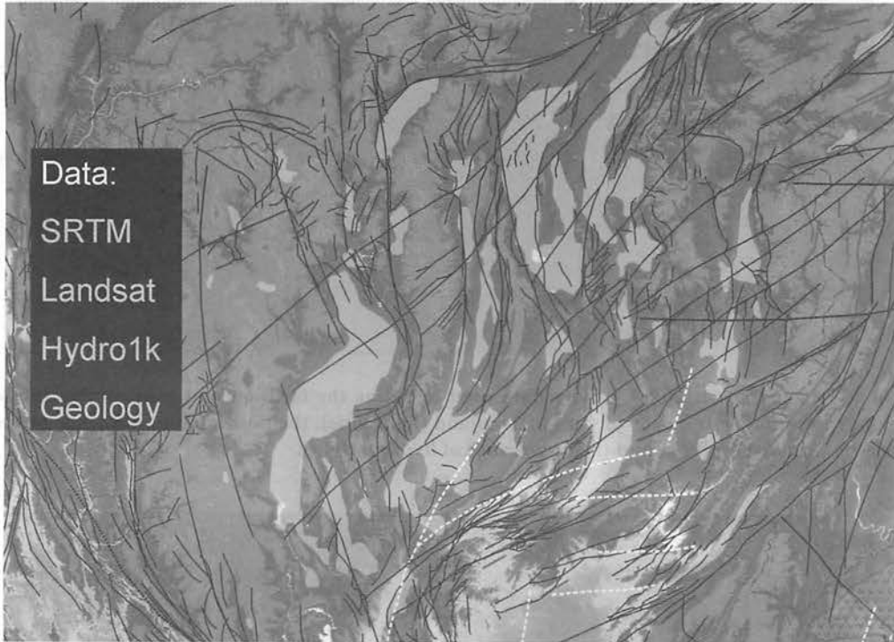
Figure 3. Datasets used to define the location and geometry of the onshore Tertiary intra-cratonic rift basins in Thailand (mauve), and the position and influence of pre-rift basement fabrics.
