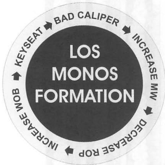
Figure 8: Drilling practices that lead to the formation of keyseat.
