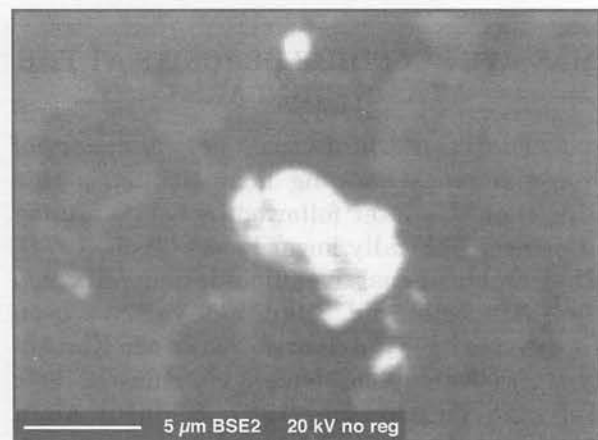
Figure 6. Gold grains infilling cavity in quartz. Sample Tc5(b), Bukit Botol.
