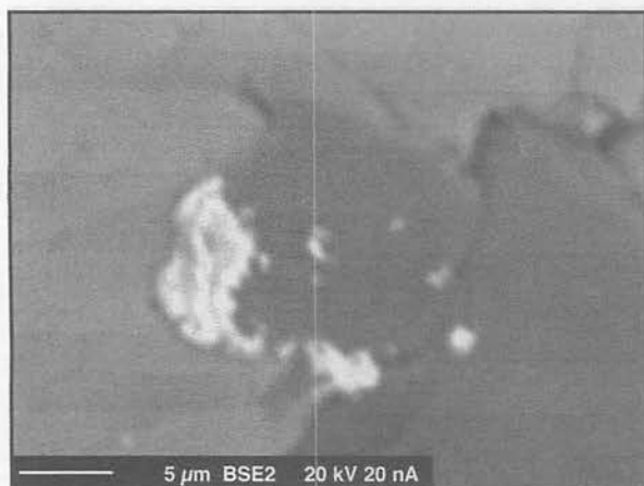
Figure 8. Gold grains (white) distributed at cooler grain boundary between barite (light grey) and pyrite (dark grey). Sample Tc7, Bukit Botol.
