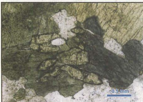
Figure 2. Anhedral sphene associated with hornblende in the Perhentian Kecil syenite.
