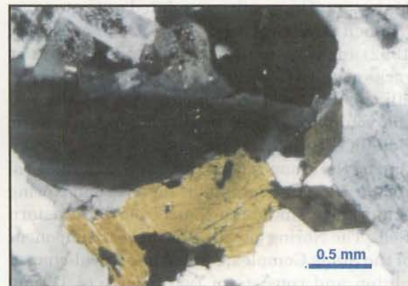
Figure 5. Two perfectly euhedral sphene crystals in the Noring granite associated with hornblende.
