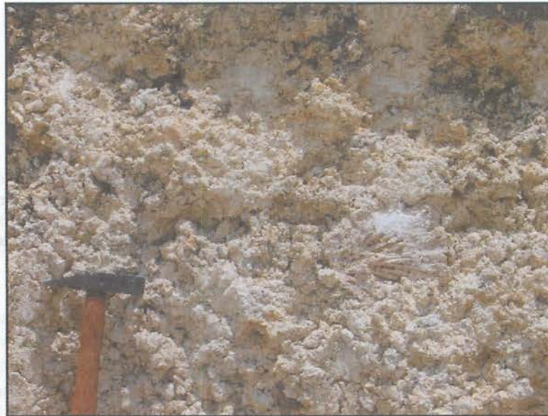
Figure 1. Porous and loosely cemented limestone with oil stains (dark patches) and coral fragments (centre right).
