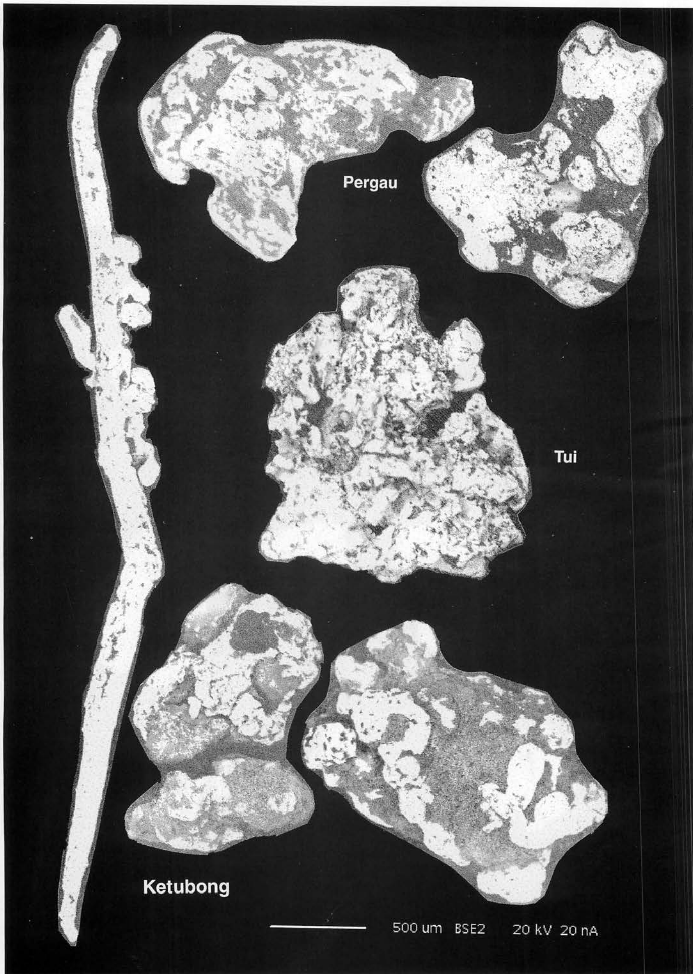
Figure 3. Scanning Electron Microscope (SEM) photomicrographs of larger alluvial gold grains from the Pergau, Tui and Ketubong areas.
