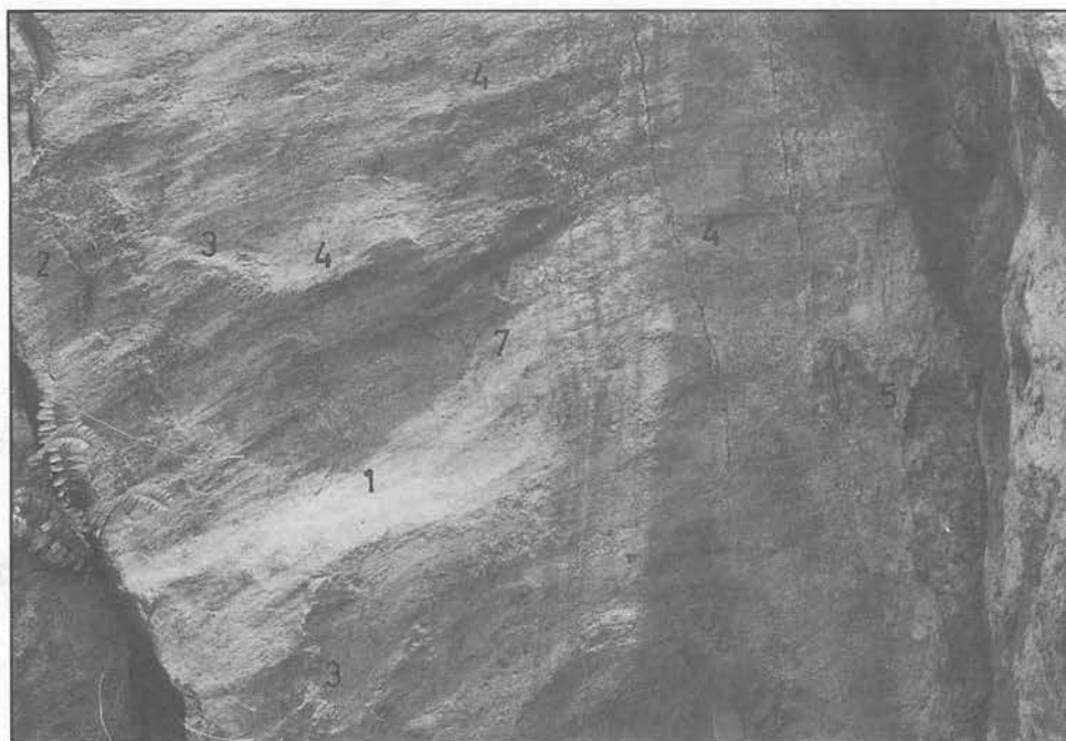
Figure 4. Displacement markings on a 310/80 slickensided fault plane through granitoid at Sri Damansara. The crescentic gouge (1) is approximately 20 cm across. Other markings for left-lateral slip are (2) accretion spalls, (3) accretion steps, (4) elongated fault roche moutonnee, (5) pluck step, (7) polished stoss sides of risers and ramps.
