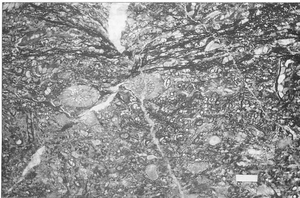
Figure 6. Photomicrograph of bryozoan limestone (scale bar = 0.1 mm)
