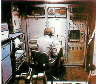
Schlumberger engineer at work with the Cyber Service Unit system inside a wireline logging Unit
