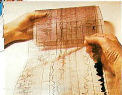
Cyberlook, an interpreted log prepared at the wellsite by the CSU computer.
