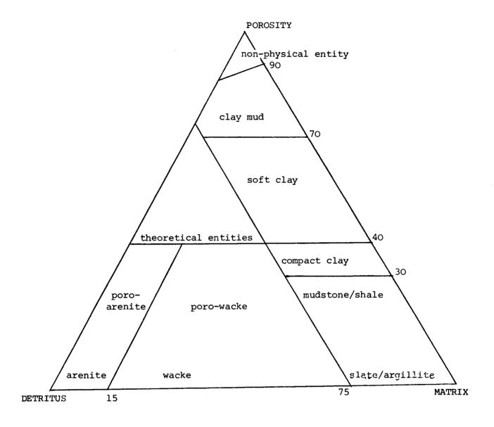
Fig. 1. Ternary diagram for the classification of porous rocks.
