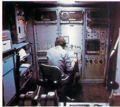
Schlumberger engineer at work with the Cyber Service Unit system inside a wireline logging Unit
