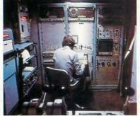
Schlumberger engineer at work with the Cyber Service Unit system inside a wireline logging Unit
