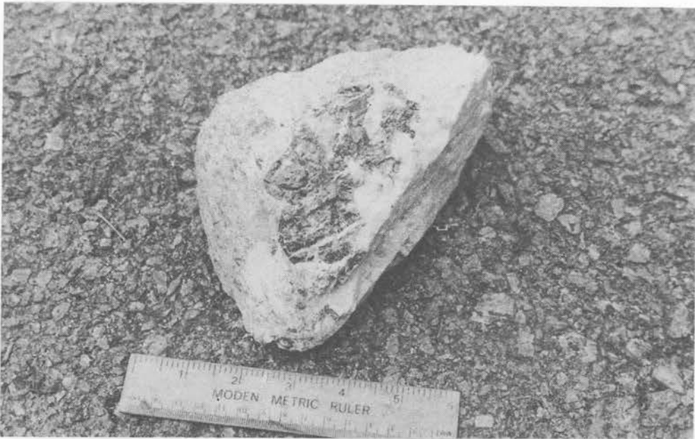
Plate 2. A fragment of cassiterite-bearing rock showing coarse-grained fractured cassiterite in contact with vein quartz on one side (right) and with altered granite on another side (left).
