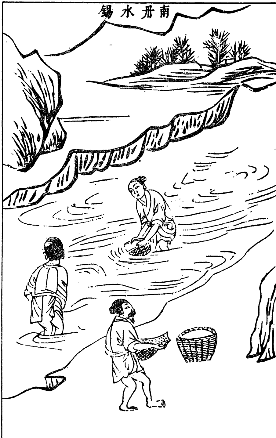
Figure 1: Recovering tin ore from the river at Nan-tan, Kwangsi.
