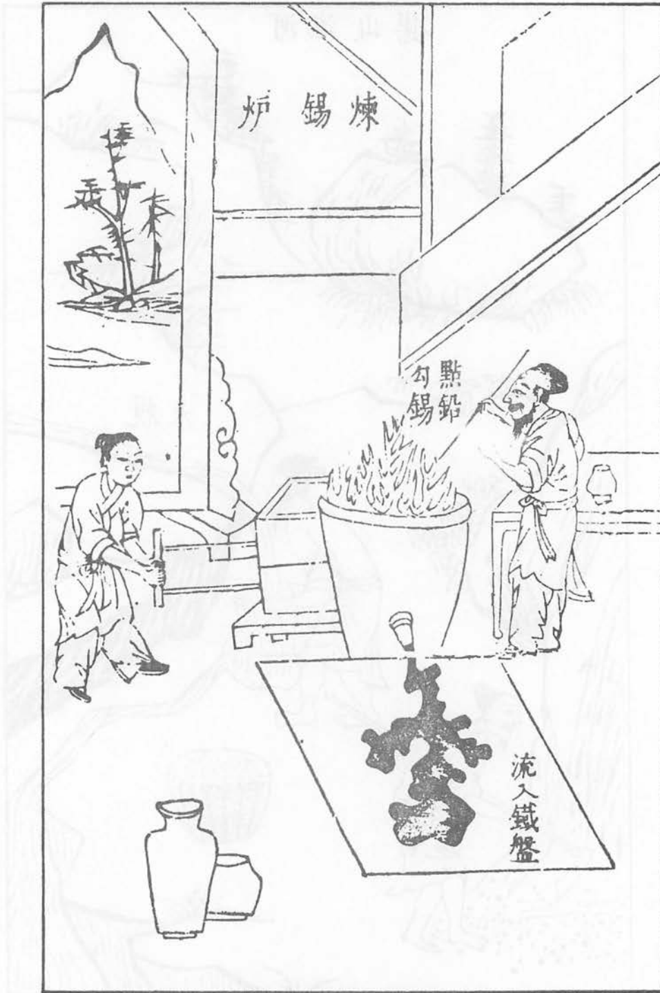
Figure 3: Smelting tin ore with the addition of lead.
