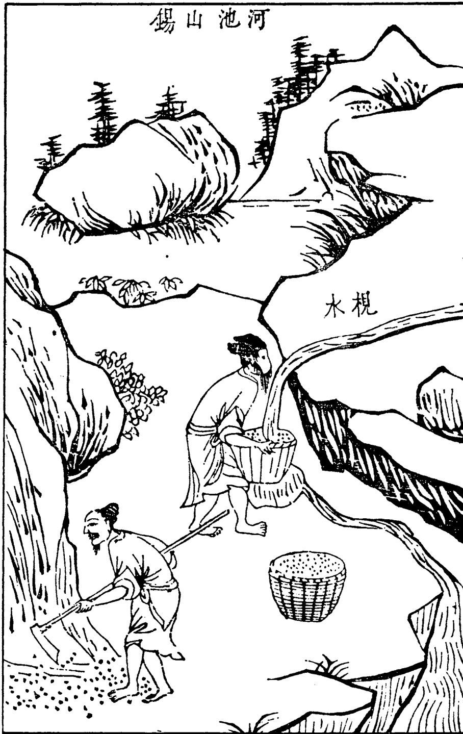
Figure 2: Concentrating mountain tin ore by washing, Ho-ch'ih, Kwangsi.
